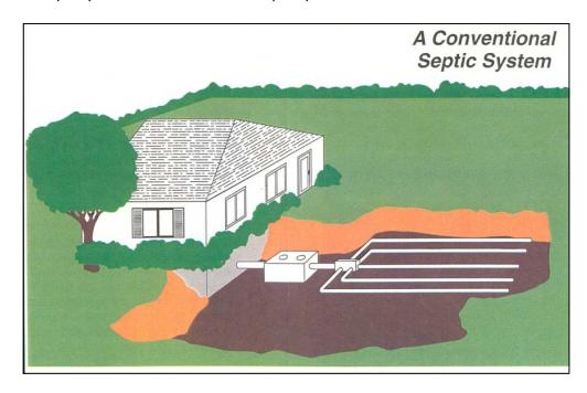
A septic system consists of a septic tank, and a drainfield, all connected by pipes, called lateral lines.
